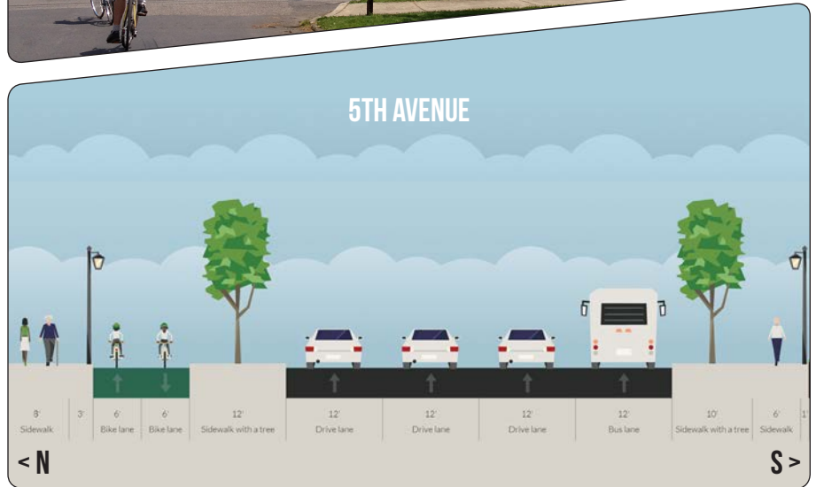
TOP: Highlawn is one of the few neighborhoods with share the road signs that are part of the PATH network. BOTTOM: Adding a cycle track on 5th Avenue for pedestrians and cyclists might improve connectivity between Highlawn and Marshall University. (Cross section made with streetmix.net.)
